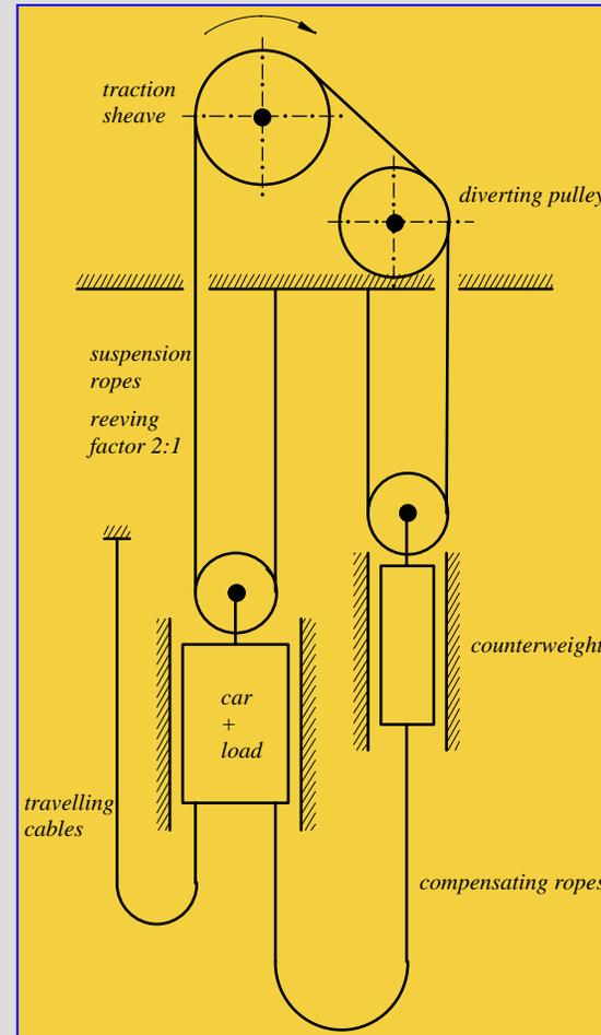
Building elevator roping configurations
