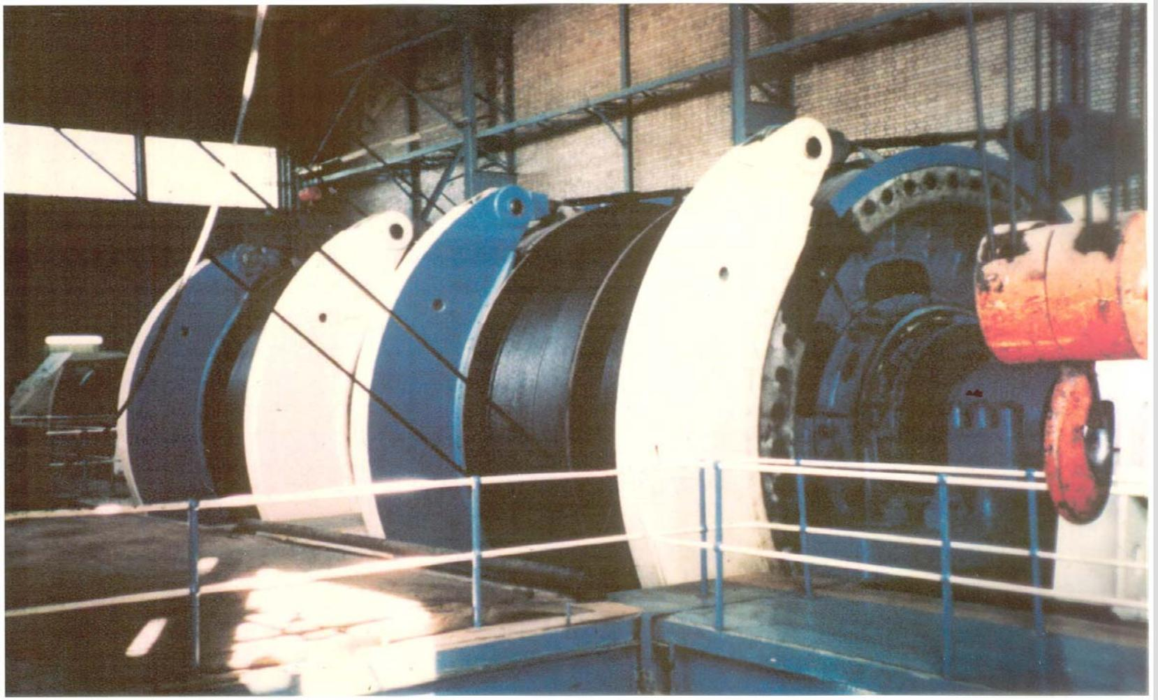
Double-drum Blair Multi-Rope winder with twin rope compartment drums
