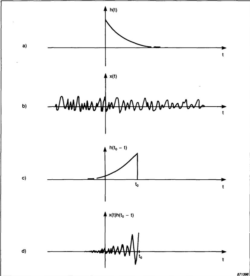
Fig. A.1. a) impulse response of a simple lowpass filter  $h(t)$ ,
