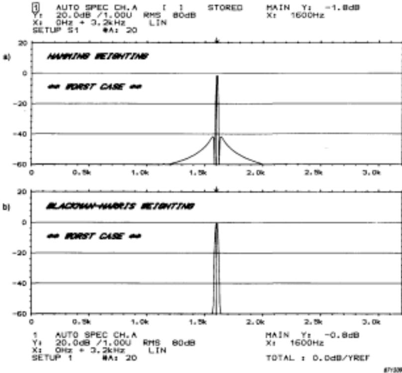
Fig. E.1. The "worst case", when analysing a sinusoid using a) Hamming window and b) Blackman-Harris window
