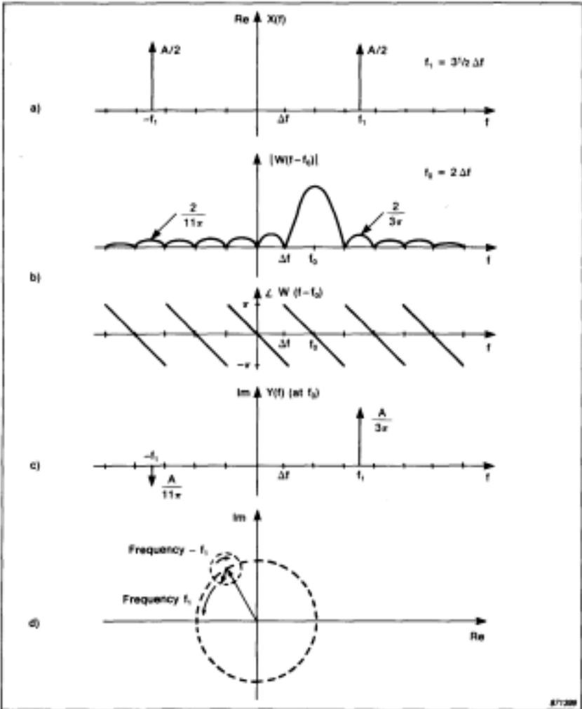
Fig. A.5. a) Spectrum of input time signal  $x(t) = A \cos(2\pi f_1 t)$ ,  $f_1 = 3/2 \Delta f$ ,
