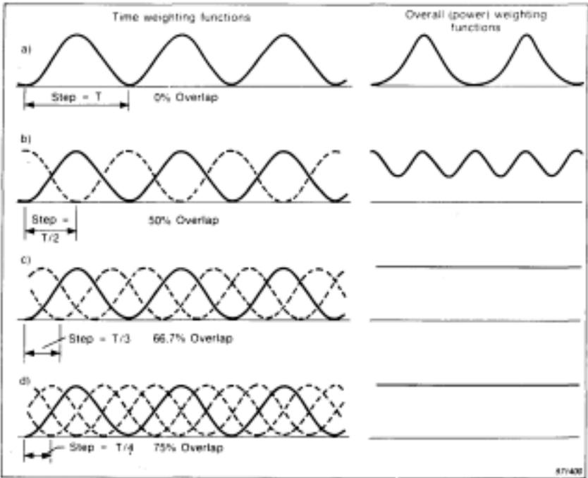
Fig. C.4. Overall weighting functions for overlapping Hanning windows
