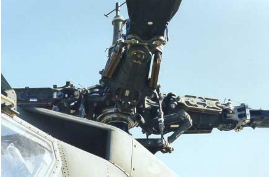
Figure 4. Main Rotor Hub
